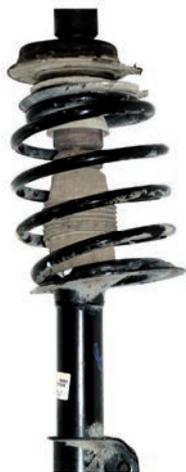
*Correctly fitted top plate*
