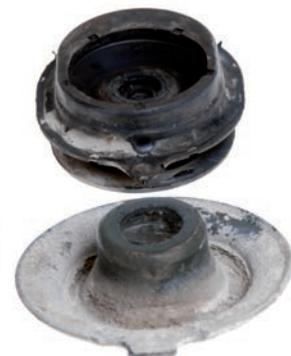
*Correctly aligned top plate & bearing*
